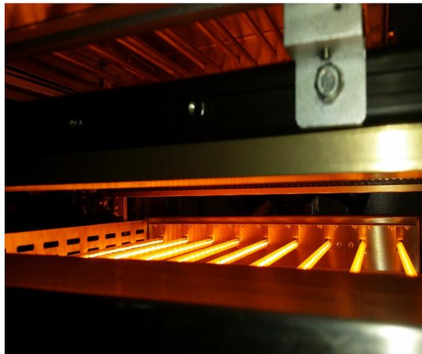
Fast reacting quartz IR preheater as standard options ensures precise preheating and flux activation before soldering.
