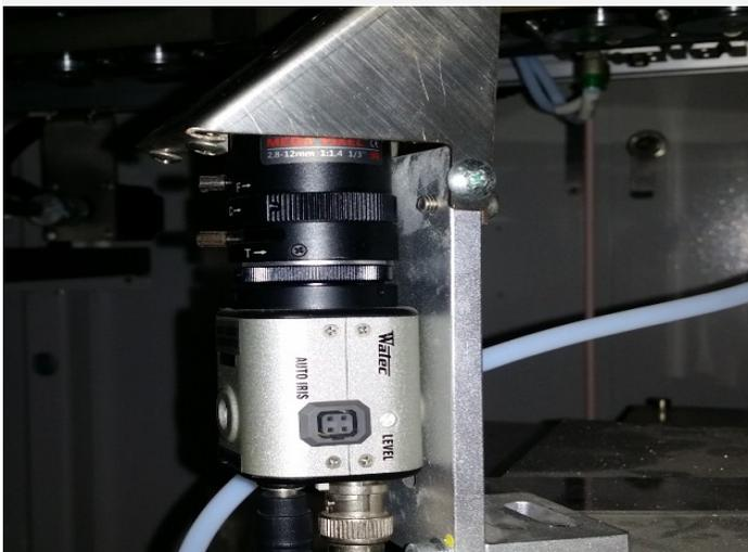
Live viewing of the soldering can assist in the process setup and continuous monitoring throughout the process. Both video and still images can be acquired from the software for archiving.
