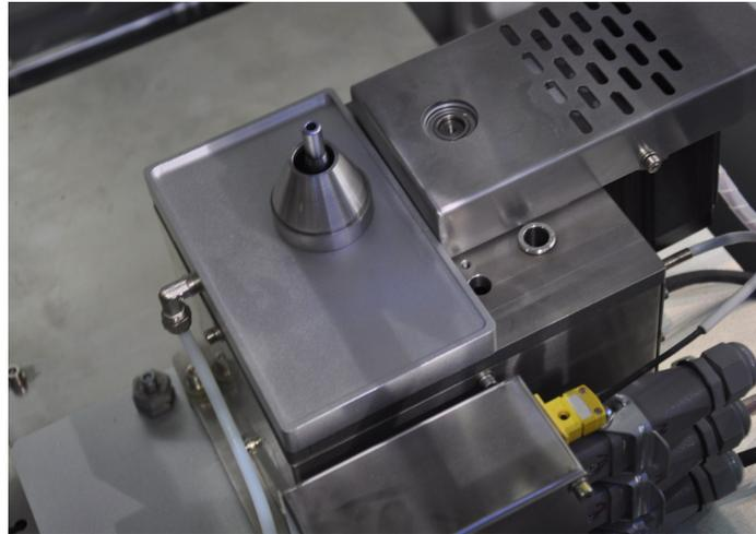
The nozzle design allows for quicker changeover times. The entire assembly can easily be removed for maintenance or allow for quick removal of the tip for changing to a different size.
